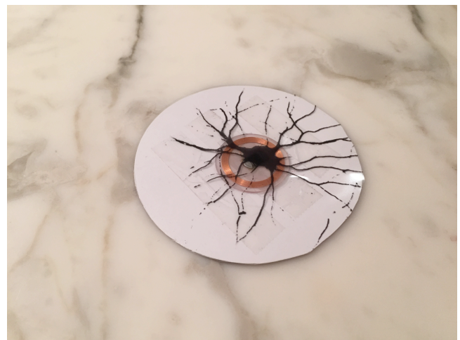
Figure 13. MiFare Classic (13.56MHz RFID/NFC) As used in project prototype
